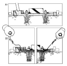
Diagram A illustrates the use of grout surcharge to ensure complete filling under a base.
